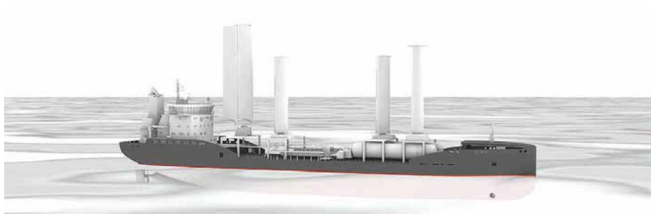
Conceptual image of wing sails (left), suction wings (centre) and rotor sail (right) on one tanker. The wing sail improves sailing performance at higher speed and during upwind legs; the suction wings improve general performance on a small deck footprint; the rotor sail enhances sidewind and downwind performance
