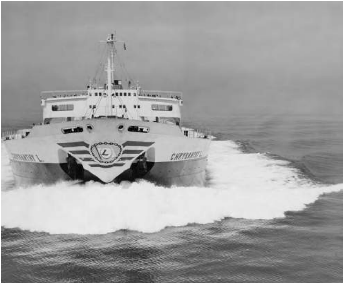
The world’s “fastest super tanker”: The “Chrysanthi L.” was built in the Kawasaki shipyards for a company under the management of Costas M. Lemos, in 1955. The vessel’s impressive capacity of 39,000 dwt and speed of around 18 knots captivated the global shipping community’s interest.
