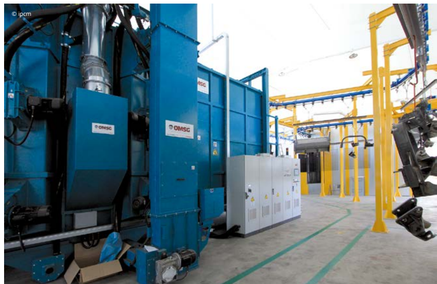
The two units performing chemical (left) and mechanical (right) pre-treatment on light-duty metal components and the Tunnelblast shot blasting machine installed in 2023.
