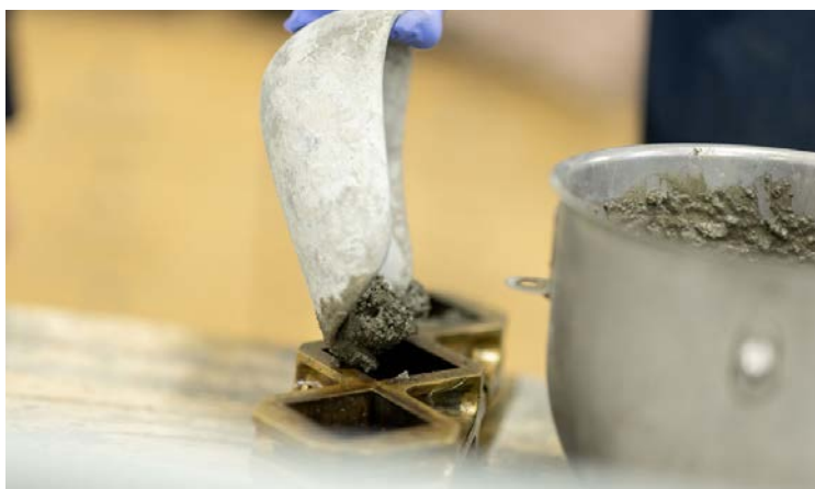
The mixture is then put into cement mortar cubes cast in moulds.
