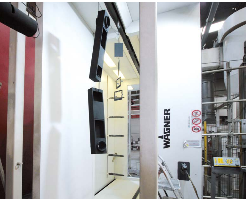
Automatic application of Interpon powder coatings in a Wagner booth.
