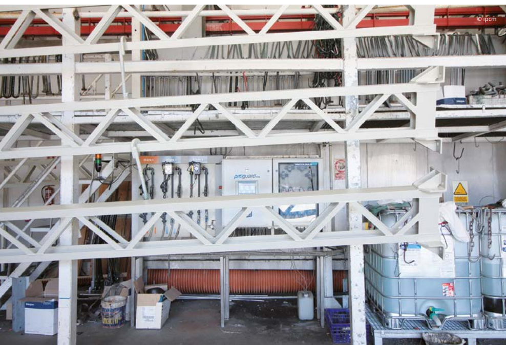
Galvanised parts undergo a chemical pre-treatment process with a nanotechnology passivation stage provided by Proquimia (Vic, Barcelona, Spain) to promote paint adhesion and improve the substrate's corrosion resistance.
