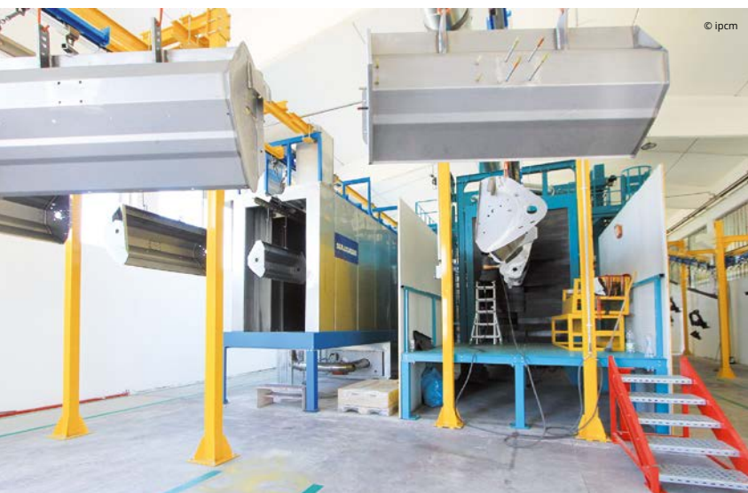
The two units performing chemical (left) and mechanical (right) pre-treatment on light-duty metal components and the Tunnelblast shot blasting machine installed in 2023.
