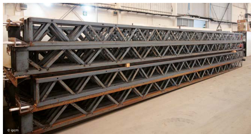
Sections of railway electrification poles awaiting finishing with the Duplex system (hot-dip galvanising + powder coating).
