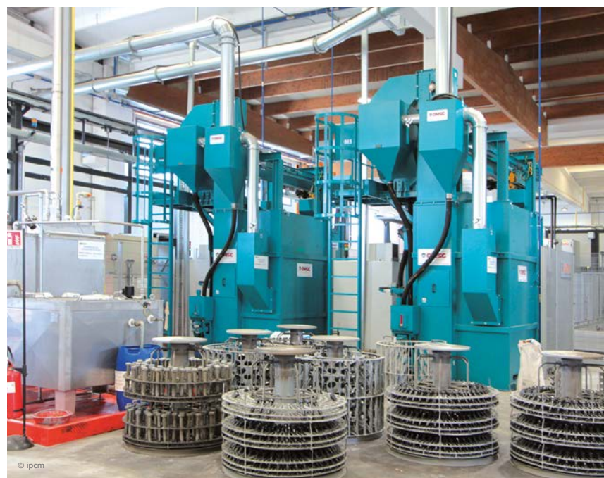
The chemical pre-treatment tanks and the two Capri-type cluster shot blasting machines from OMSG.
