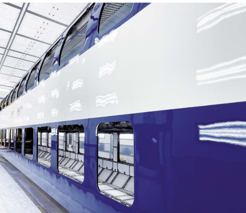
Three colours can be applied on the wagons' exteriors: white, blue, and red. The booth is designed to flexibly coat rolling stock in any size.
