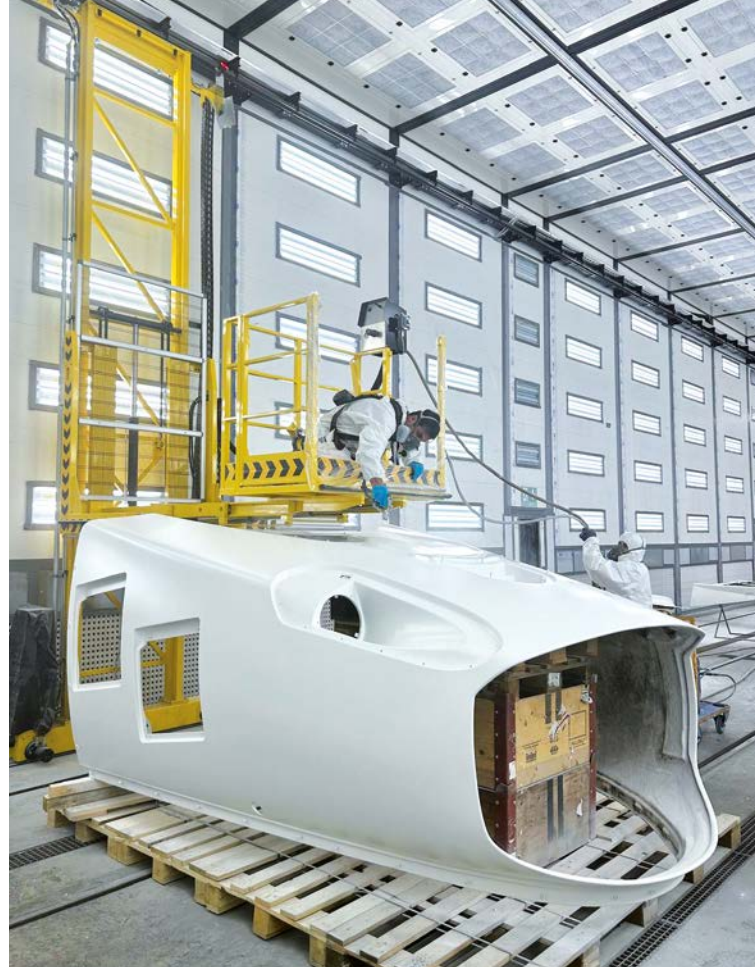
Three colours can be applied on the wagons' exteriors: white, blue, and red. The booth is designed to flexibly coat rolling stock in any size.
