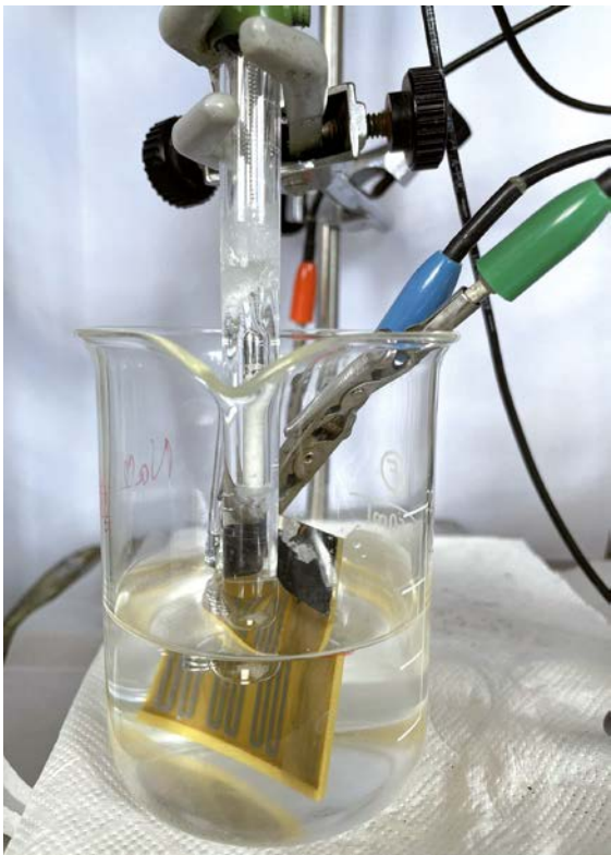
Figure 6 - EIS measurement on resistometric sensors to ensure data comparability.
