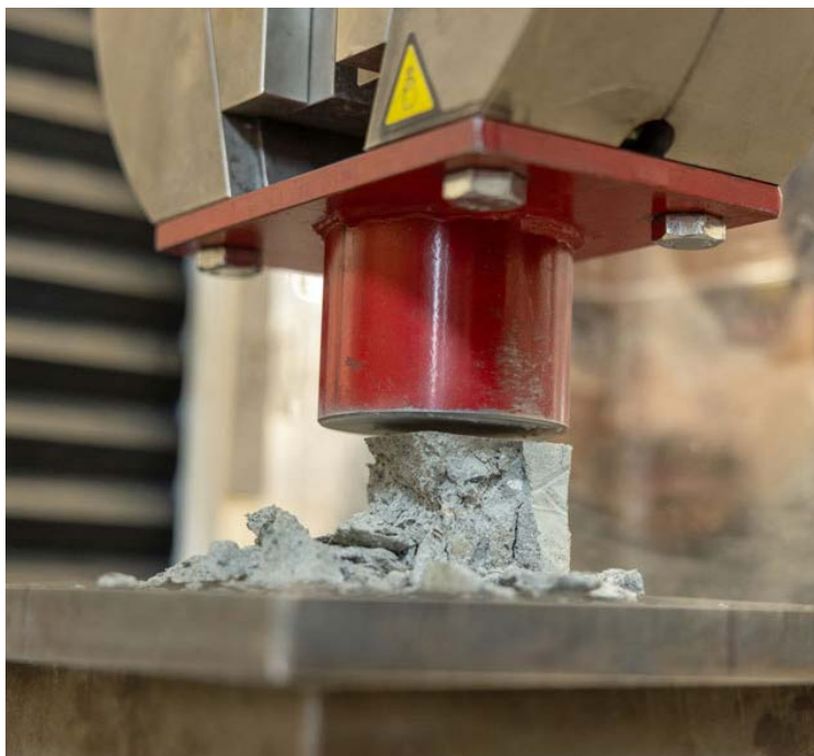
The cubes are tested after 28 days of curing under standard curing conditions.
