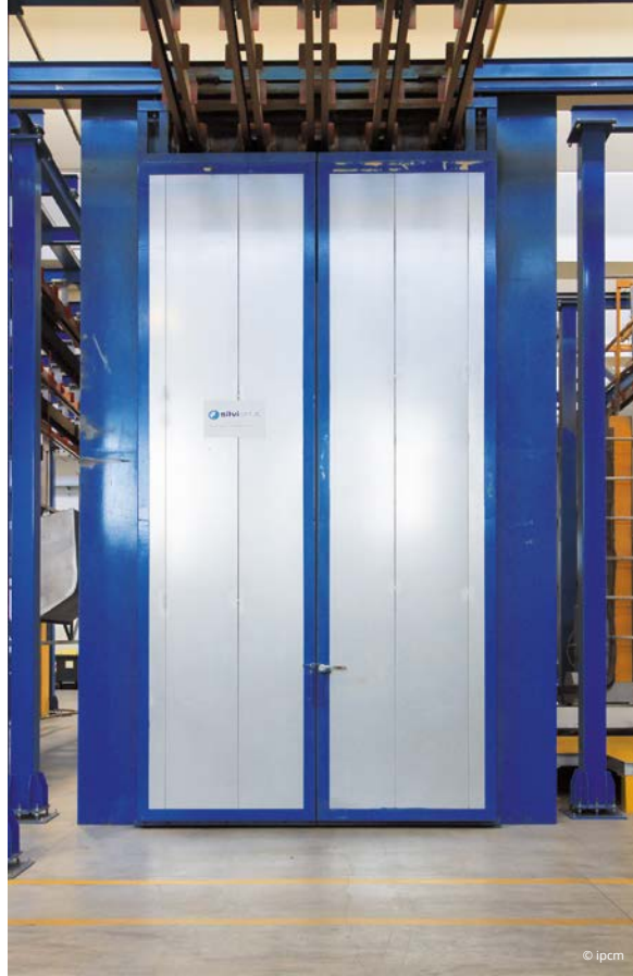
The Gema booth equipped with 12 guns (6+6).
