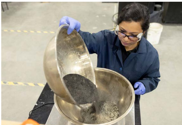
Killam doctoral student Rubaiya Rumman performs tests to find the optimum replacement level of cement with wood fly ash to produce green concrete.
