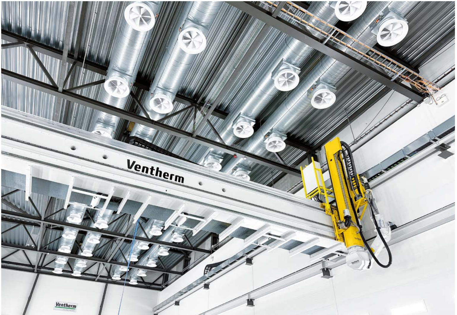
The robot's gantry system comprises two parallel rails mounted on the walls, supporting a crossbeam that moves horizontally along the X-axis.
