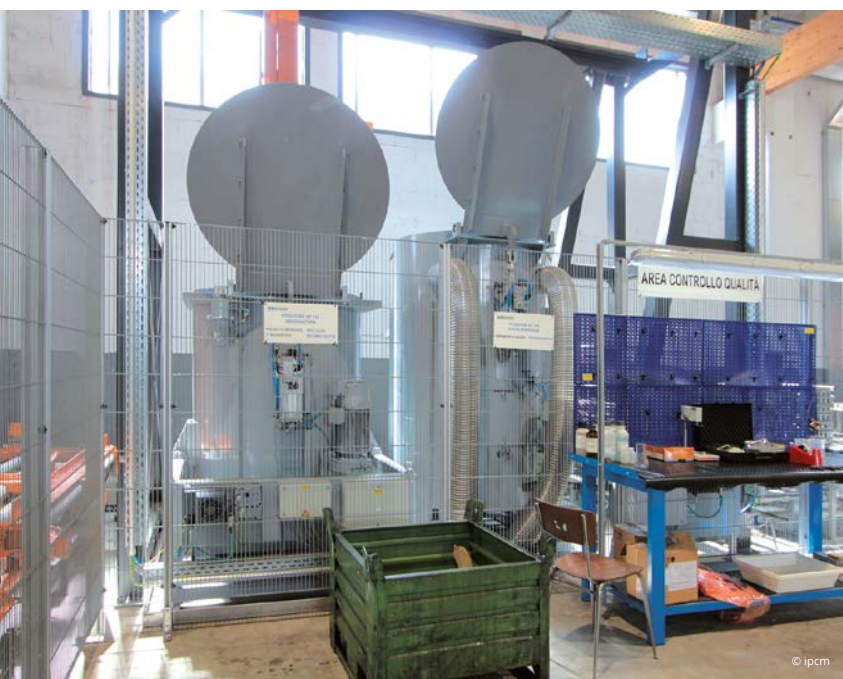
The chemical pre-treatment tanks and the two Capri-type cluster shot blasting machines from OMSG.
