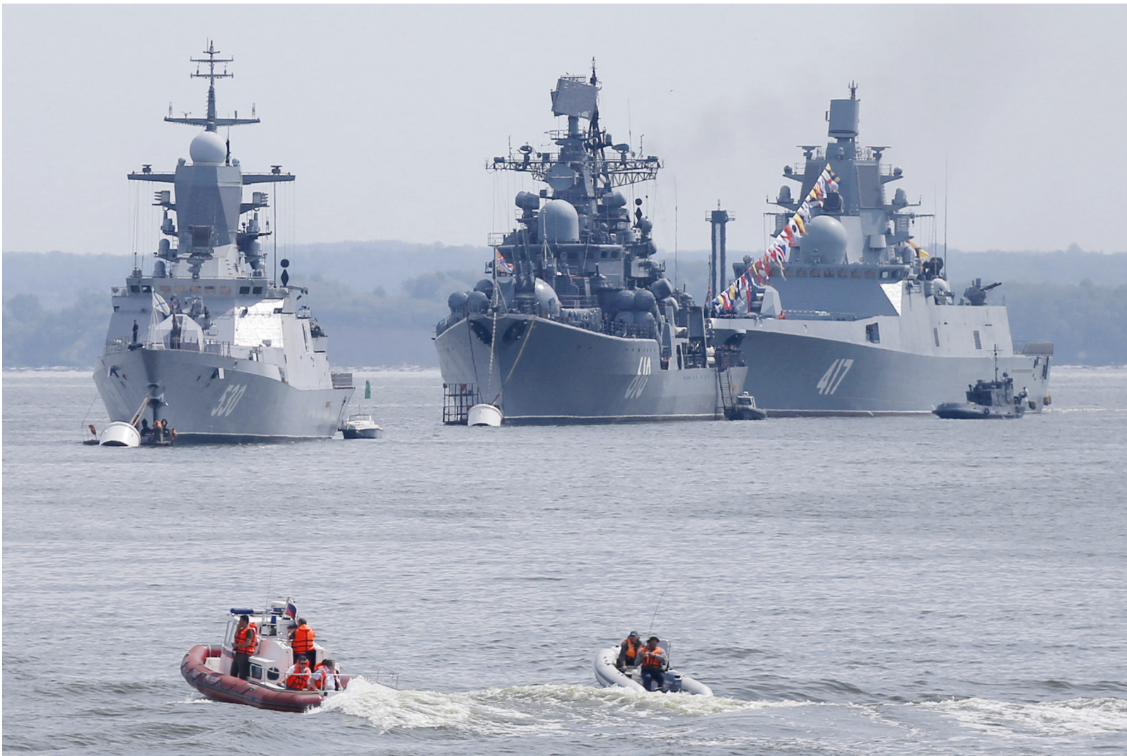
The Projekt 20381 corvette Steregushchy (530; left) and the Projekt 22350 frigate Admiral Gorshkov (417) possess latest Russian naval technology. Note the latter's four-face Poliment 5P-20K multifunction S-band Active Electronically Scanned Array (AESA) radar. Both ships are pictured here together with the 1980-era Sovremennyy class destroyer Nastoychivyy (610) in the Kaliningrad region. (Photo: Russian Navy)
