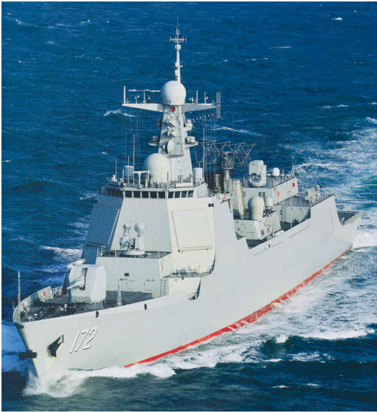
The multifunction AESA radar based on the indigenously developed Type 346/348 DRAGON EYE active phased array radar fitted to Luyang III class (Type 052D) guided missile destroyers may be as powerful as the US AN/SPY-1 system. (Photo: PLAN)
